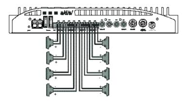
speaker connections for bridged configurations
